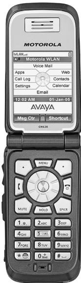
**Figure II-2:** An integrated cell phone/WiFi phone.
